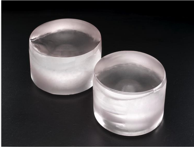
Pictured Above: 130kg and 100kg boule grown in GT's Salem, MA Factory
