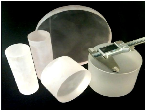
Pictured Above: 130kg and 100kg boule grown in GT's Salem, MA Factory
